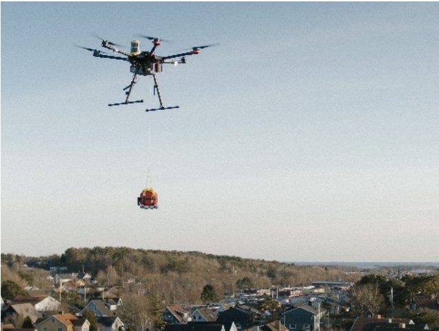
Fig. 2 – AED equipped UAV, provided by Everdrone AB
